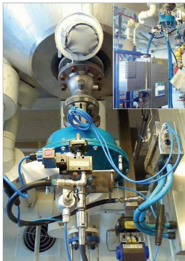
Above: SchuF valve with integrated Mettler Toledo ReactIR™ FT-IR probe installed at the outlet of a reactor. The probe is connected to an online reaction-monitoring instrument.
